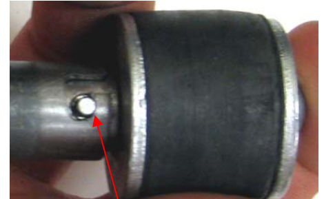
Bayonet Mount Pin must engage the L-shaped slot.
