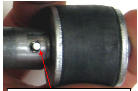
Bayonet Mount Pin must engage the L-shaped slot.
