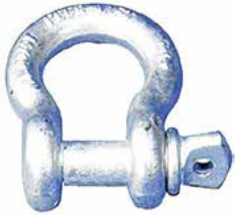
PEERLESS SHACKLES • Hot dipped galvanized to ASTM A153 • Proof load at 2 times the working load limit • Ultimate load at 5 times the working load limit • Meet or exceed FED SPEC RR-C-271D requirements • 5/16", 3/8", 7/16", 1/2", 5/8", 3/4", 7/8", 1", 1-1/8", 1-1/4", 1-3/8", 1-1/2", & 2"
