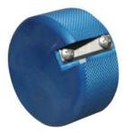
**Chamfering** tools are designed to make a bevel on the outside edge of a pipe end for socket fusion / electrofusion. This Chamfer allows heater faces and socket fittings to be easily pushed onto the pipe end.
