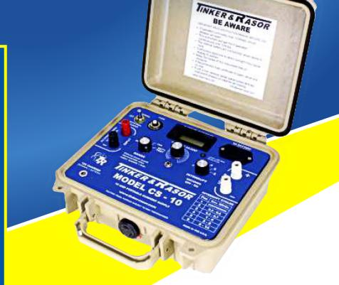
The CS-10 portable current supply is an ideal DC current source for many cathodic protection corrosion maintenance tests. Commonly used for determining current requirements for cathodic protection or impressing current on an underground structure for assisting in locating electrical contacts with foreign systems such as underground utilities.
