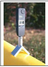
On pipe > 2" position tool on pipe as shown above. On pipe < 2" rotate the tool 90° & position on pipe using the small "V" slot.
