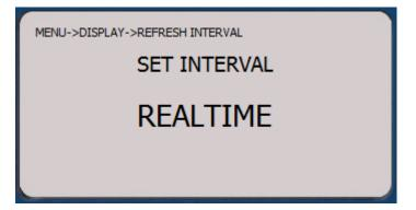
If a high update rate is not needed the interval can be extended to conserve battery life. To adjust the refresh intervals in seconds, use the Arrow Keys and press SELECT. The interval can be set to a maximum of thirty seconds.
