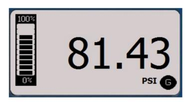
If you would like to focus on a couple different engineering units or prevent certain users from using an unapproved choice for calibration, units can be locked or unlocked under Units in *Program Mode*.
