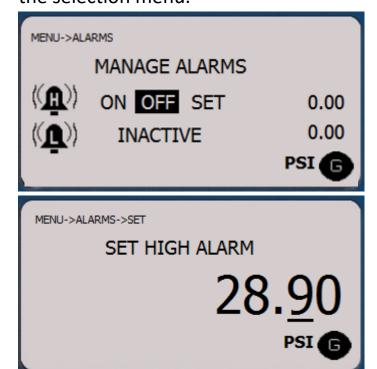
Once the alarm setpoint has been reached the high or low alarm icon will show on the display and background color will change to red to indicate an alarm status.
