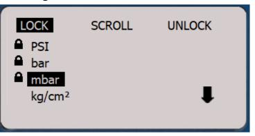
Use the right or left ARROW keys to highlight LOCK, SCROLL, or UNLOCK. Use the up or down ARROW keys to either LOCK, SCROLL, or UNLOCK the engineering units, depending on which function is highlighted.
