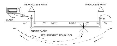
Set the Transmitter to fault mode by pressing and holding the frequency button for 10 seconds. When released the DFF symbol on the LCD will be displayed.
