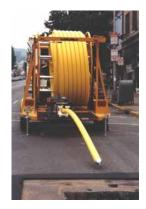
PLCS trailers are only as long as a pick-up truck (less than 17' x 8'). They are invaluable in tight city streets yet can also lay high volumes of pipe, at high speed, across country. The coil bay can handle PE and HDPE coils up to 54" wide x 128" OD x minimum 42" ID.
