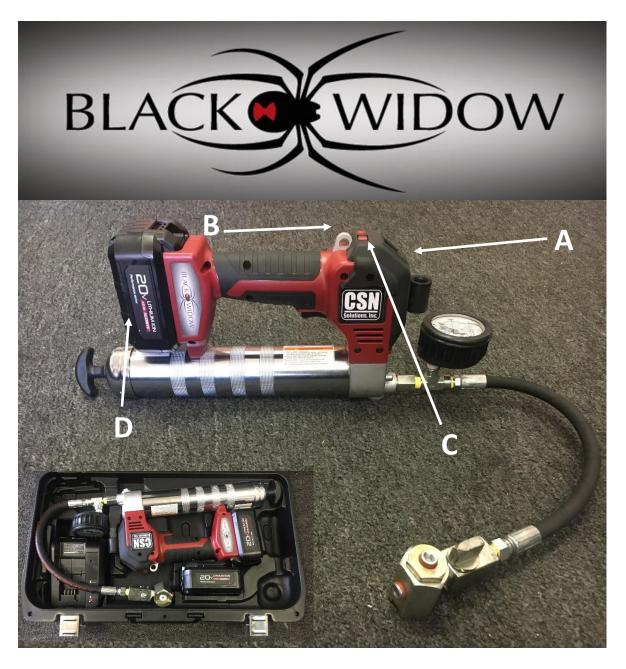
The new 10,000 psi, 20 Volt, 4 amp battery operated hand gun comes with a 15K pressure gauge, tee, 14" hose, shut-off valve and a giant button head coupler. Also included is an extra 20 Volt battery, battery charger and a carrying case. Cartridge Grease Only.
