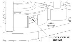
11. If adjustment is required to allow the shoe to retract further, loosen lock collar located inside lock collar housing. The lock collar screws are accessible through slots in lock collar housing. Slide launch tube to retract the shoe to the desired position then tighten the two lock collar screws.
