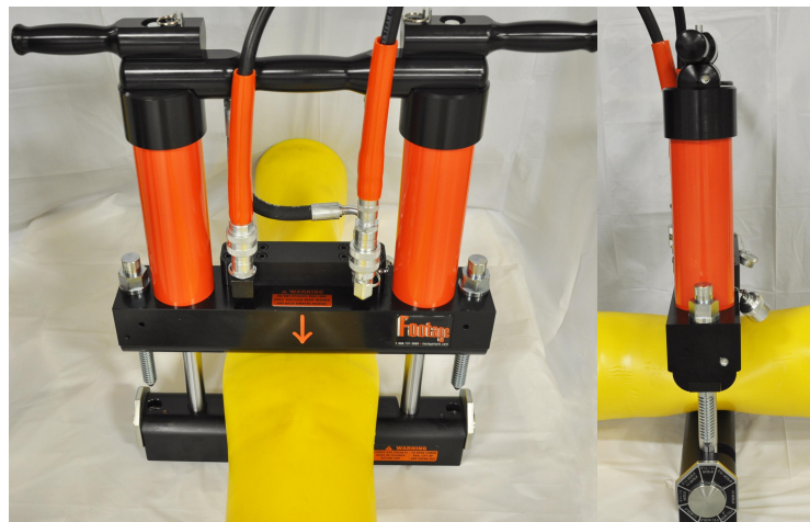
PLACE TOOL CENTRALLY ON PIPE & AT 90° TO PIPE
