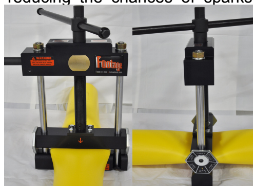
Place tool centrally on the pipe and at 90° to the pipe
